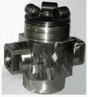
The aim of developing the new product was to replace the existing valve 2 3/8NUE  $\times$  700bar, that used in an environment of crude oil and salt water was not always satisfying the expectations of the user. The replaced valve was used mainly with the cementing unit ACF 350  $\div$  700.
