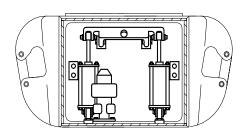
Pneumatic drive for spider elevator
