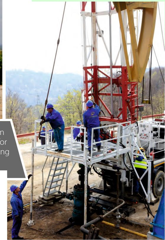
The AM12/50 mast equipped workover rig is the result of long experience in manufacturing (AM 10) and repairing of workover rigs. It is designed for intervention and overhaul of oil and gas wells without derricks, of which working depth is in accordance with 50tf hook loads, to perform the following tasks:
