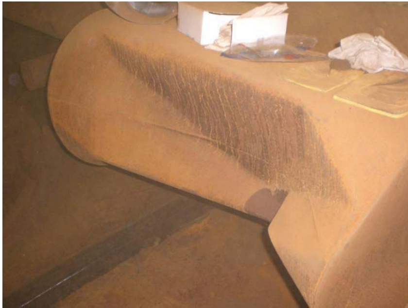
Pic 52: Massive deformation of the swivel floaters.
