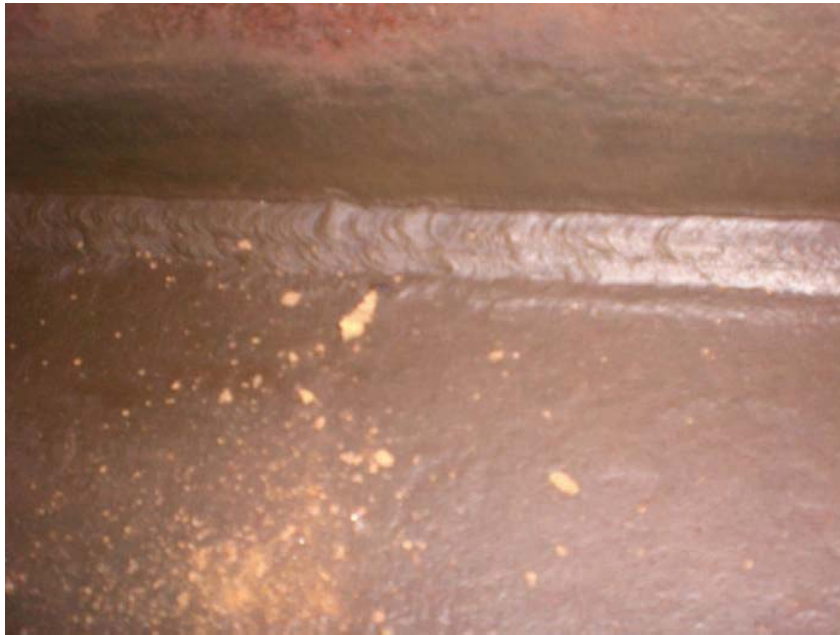
Pic 64: Undercut on the corner weld.
