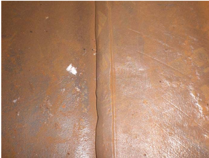
Pic 60: Heavy undercut and lack of fusion at the bottom welds.
