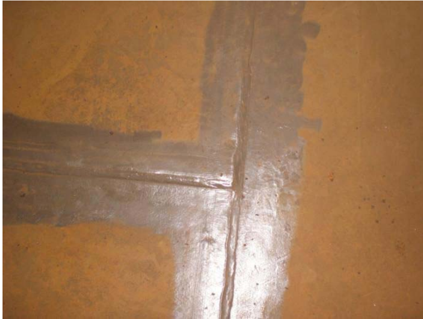
Pic 61: Undercut and underfill present on the bottom welds.
