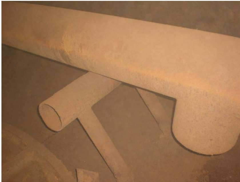
Pic 50: Outlet swivel. Support not fully welded to the bottom.
