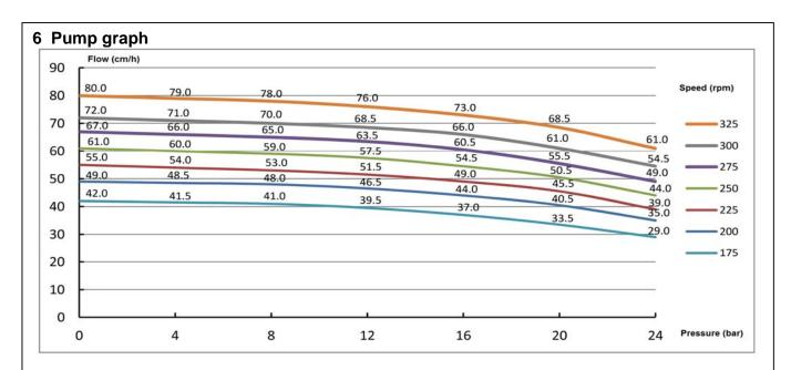
The above diagram shows theoretical performance of this pump type and provides a good orientation when selecting a pump. Actual diagram related to a specific pump serial number is built during testing on the bench stand of that particular pump and is available with the delivery documents.
