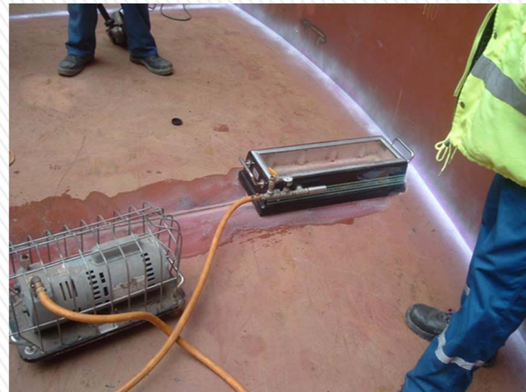
Vacuum check of welds
